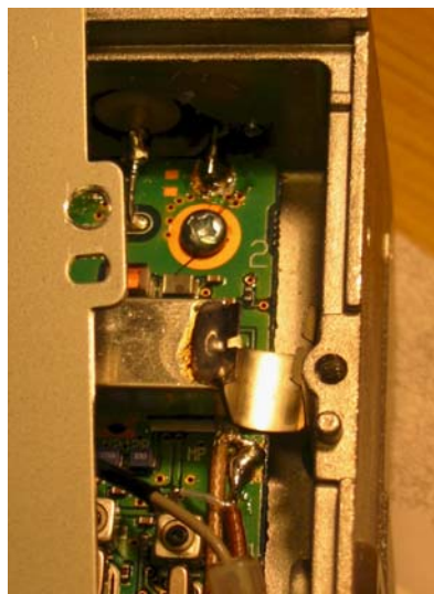
15. Prepare a thin coax cable and solder the inner conductor to the output of the balun transformer (where you removed C220 before). Use the dark color or mark it as "Mixer cable UHF" 16. Cut the shielding box at this corner to allow the coax to leave the box. Bent the cut' part up. Re-install the shielding box and solder the outer conductor of the coax to the box. (Ground and strain relief). Mark this cable as 'mixer' cable going to the IF input of IFD. 17. Prepare a second coax cable and solder to cathode of D220/D221 (showing towards shield box), 1cm distance. Solder the outer connector to the shieldig box. Use the brighter cable or mark this cable as 'filter UHF', going to output of IFD. 18. Feed both coax cables through the opening near the fan to the opposite side. 19. Connect both ends of both cables with a 100 pF capacitor and repeat step 1. The S-meter should read S8 at 70cm (when the same voltage as required for S9 before is applied) (this step may be omitted) 20. Re-install the PA unit. If necessary, add some heat conducting grease. Reinstall the thermal sensors and double check that all power-transistor screws are tight. 21. Best place to install the IFD is on the panel over the PLL unit, where you find the brackets for DSP1 and DSP2 unit. However, you cannot use the DSP2 option later.
