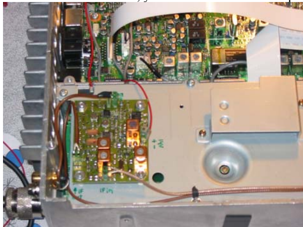
15. Prepare a thin coax cable and solder the inner conductor to the output of the balun transformer (where you removed C220 before). Use the dark color or mark it as "Mixer cable UHF" 16. Cut the shielding box at this corner to allow the coax to leave the box. Bent the cut' part up. Re-install the shielding box and solder the outer conductor of the coax to the box. (Ground and strain relief). Mark this cable as 'mixer' cable going to the IF input of IFD. 17. Prepare a second coax cable and solder to cathode of D220/D221 (showing towards shield box), 1cm distance. Solder the outer connector to the shieldig box. Use the brighter cable or mark this cable as 'filter UHF', going to output of IFD. 18. Feed both coax cables through the opening near the fan to the opposite side. 19. Connect both ends of both cables with a 100 pF capacitor and repeat step 1. The S-meter should read S8 at 70cm (when the same voltage as required for S9 before is applied) (this step may be omitted) 20. Re-install the PA unit. If necessary, add some heat conducting grease. Reinstall the thermal sensors and double check that all power-transistor screws are tight. 21. Best place to install the IFD is on the panel over the PLL unit, where you find the brackets for DSP1 and DSP2 unit. However, you cannot use the DSP2 option later.
